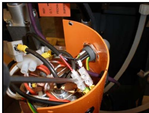
**10-** Install the new fittings and thermocouples, make sure that the tapered end of the ferrule is facing the fitting.
