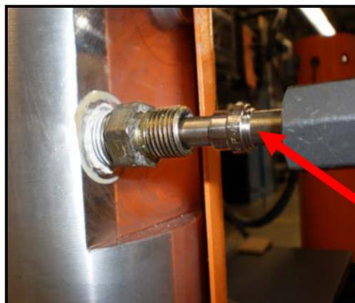
**11-** Push in on the thermocouple and tighten the ferrule locking nut while holding the thermocouple against the heater cartage. **Ensure the Thermocouple is in positive contact with the fire rod while tightening nut.** Make sure the position of the thermocouple is in the approximate 4 o'clock position on the "a" heater and 7 o'clock on the "R" heater while tightening the locking nut. Insert the thermocouple metal sheathing into the grommet approximately 1".
