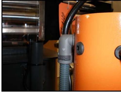
**7A-** On the G250 the original hole is closer to the top and on the back cover rather than the side. Drill new hole 2-3" from it this hole on both heaters
