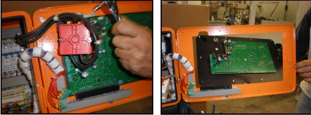
5- Insert the new panel and install using the 10 mounting nuts that you removed from the old panel.
