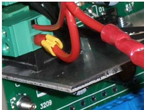
**16-** Pull the TSU harness out of the channel and, you will have to loosen the strain relief on the bottom of the console and pull the wire up into the console to reach the controller.
