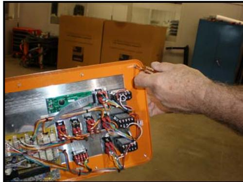
6- Reinstall the main electrical switch.
