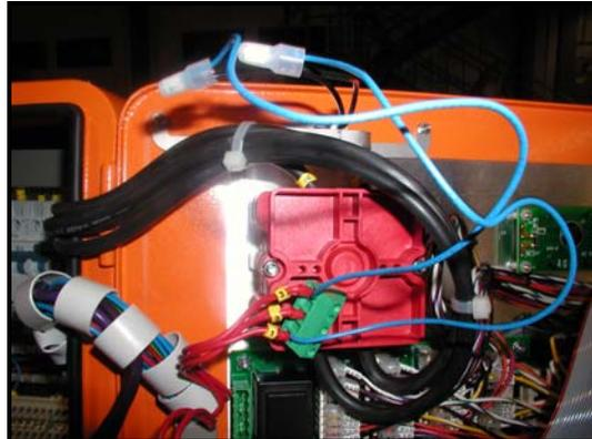
**15-** Remove either the #4 or #5 wire from green terminal block, cut of end terminal and strip wire. Insert one red wire from control power switch into green terminal block where the red wire was removed. Connect the other red wire from the control power switch with the wire that was removed from green terminal block. Reinstall green terminal block to control board.
