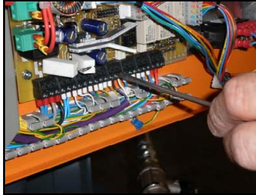
**14-** Connect the wires from light on panel to terminals 1 and 3 on green terminal strip.
