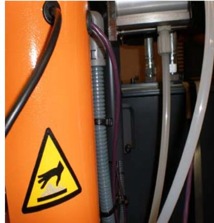
**9-** Remove the thermocouples from the heaters and remove the fittings. Disconnect the wire from the connector inside the heater and pull the wire out, discard these parts.
