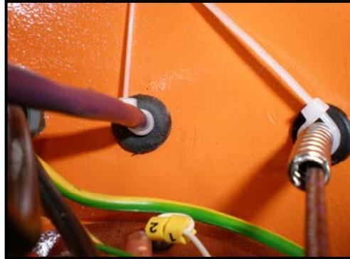
**13-** Install the power strip onto the new panel. You may have to reposition the wires in the channel to match the positions on the connector. Remove the wires 15 and 16 counting from left to right. Remove the cable that contains these wires and from the channel and reconnect wires to hose controller
