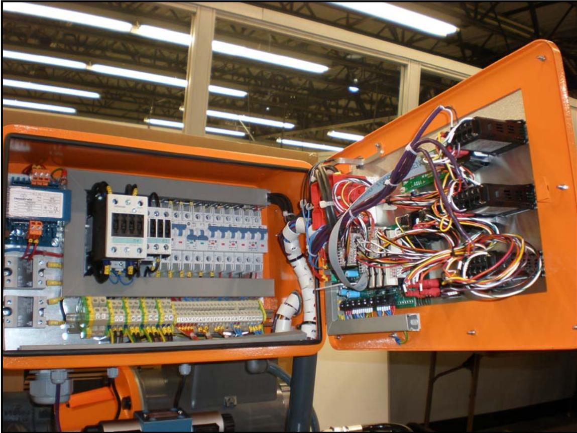
**19-** Remove the cover from the reversing switch and move the center wire on the “R” side reversing switch to the end position.
