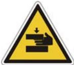
***To prevent serious harm by crushing or loss of limbs, do not work with the unit without the safety guards installed on all moving parts. Make sure that all of the safety protections are correctly reinstalled after all repair or maintenance work is completed.***
